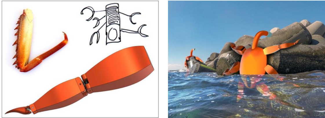
Fig. 4: (a) Biomimic Rock Crab Legs, (b) PowerCrabs in a Future Deployment
