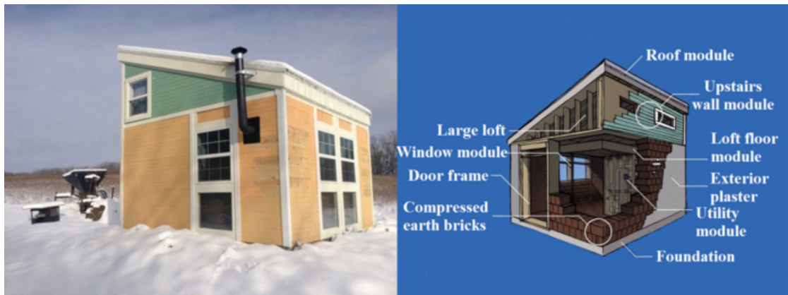
Figure 4. The OSE Microhouse project and its building modules Source: Adapted from Open Source Ecology, 2018
